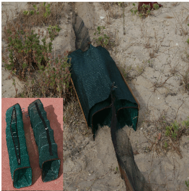
Fig. 1. Pair of funnel traps located either side of a drift fence with a shade cover. Insert: funnel traps showing zipper and shape.
